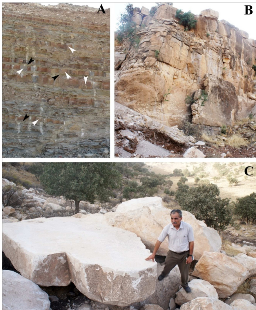
Figure- 2:A. Section of Sandstone beds (Tanjero Formation) near Germany Village-Sulaimani, the white arrows indicate sandstone beds and the black one indicates the greenish marlstone. B. Section of limestone beds (Pila Spi Formation) in Quarry near Blkan Village. C. Block of white limestone prepared to be transported to marble's Factory in Sulaimani City.
